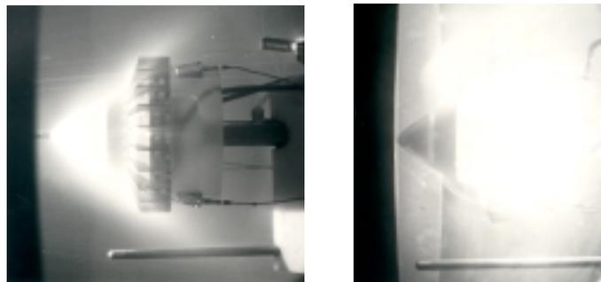
Figure 8- Open shutter photographs of the luminous Mach 7,8 airflow past the inlet with the magnetic field off, left, and on, right. Flow is from left to right.
